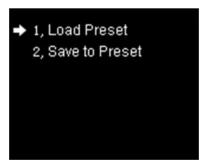
In the submenu, 16 preset parameters can be saved, and every preset parameter includes all parameter information of image output (signal source, PIP, scaling, clipping, picture adjustment), users can also directly load the saved preset parameter to display the image according to needs, and don't need to set up all parameters again.
