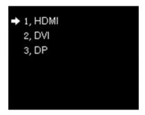
Enter the EDID setting interface of "HDMI" or "DVI" or "DP". Rotate the knob to select conventional resolution; or set width, height and frame rate by knob in the option of "Custom".
